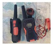
We've also used the rugged AM1055 FLT radios from Cobra featuring a floating & waterproof (IPX7) design.
